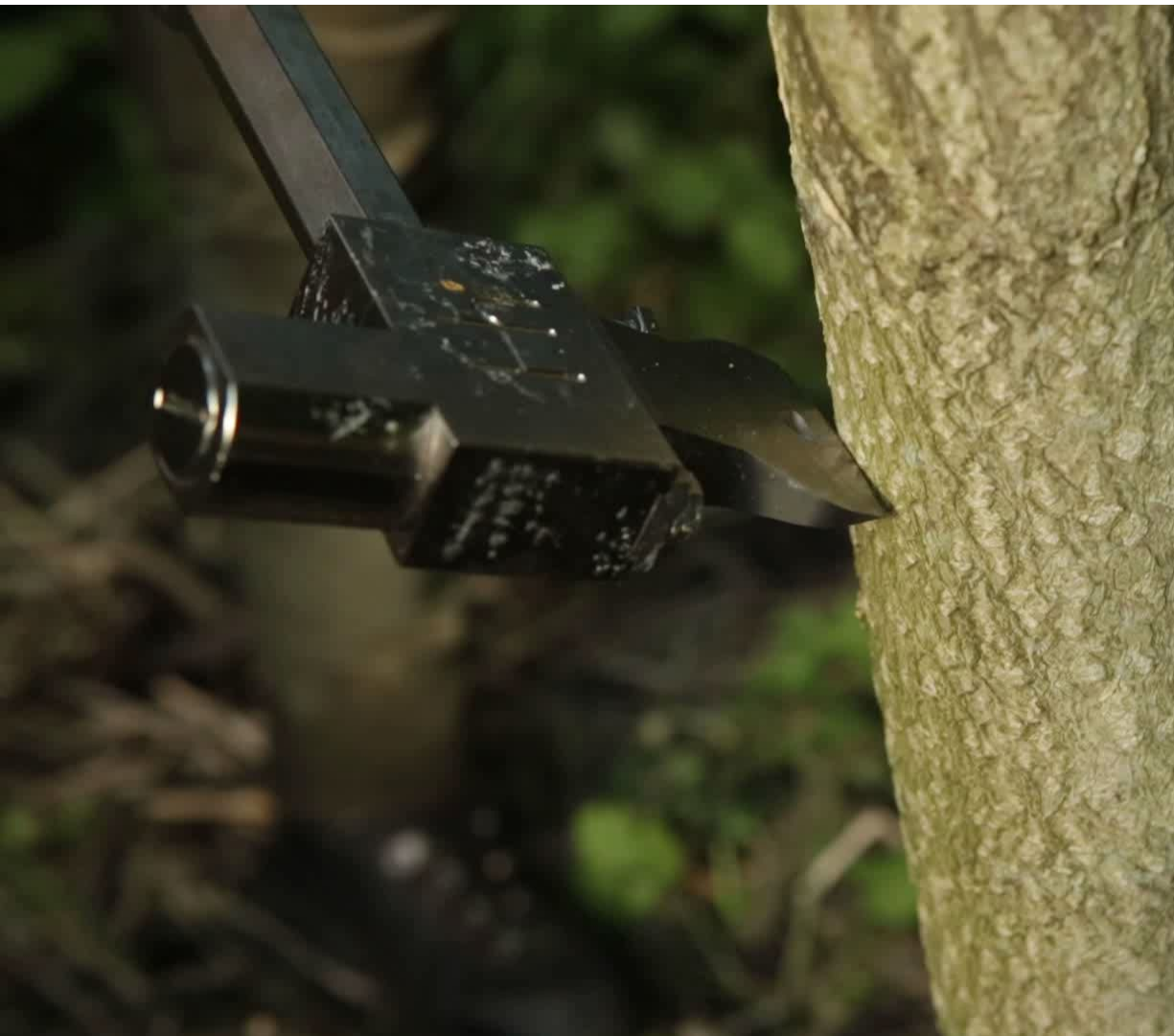
Hypo-Hatchet: developed for application of liquid herbicides
